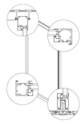
B. Identify Intermediate Panel (skip if 2 panel door) - This panel will have two interlock stiles.
