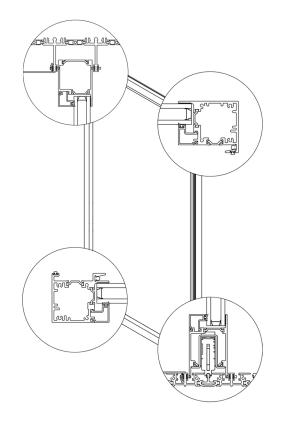
B. Identify Intermediate Panel (skip if 2 panel door) - This panel will have two interlock stiles. Position the panel so the glazing stops facing the exterior. With half the panel overlapping the lead panel, insert the panel into the next track, lifting while pivoting the door to the next threshold track. Adjust rollers to match sightlines and with previous panel. Repeat for each intermediate panel.
